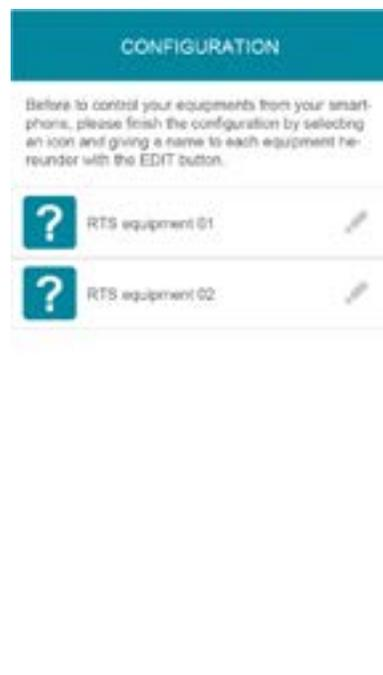
**[A]** To complete your installation, you need to customise the registered equipment. Click on the pencil positioned to the right of the equipment to be customised.
