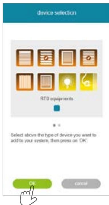
**[D]** Select the type of product that you wish to add to the installation: RTS motors/ actuators or Philips Hue lights, then confirm by pressing
